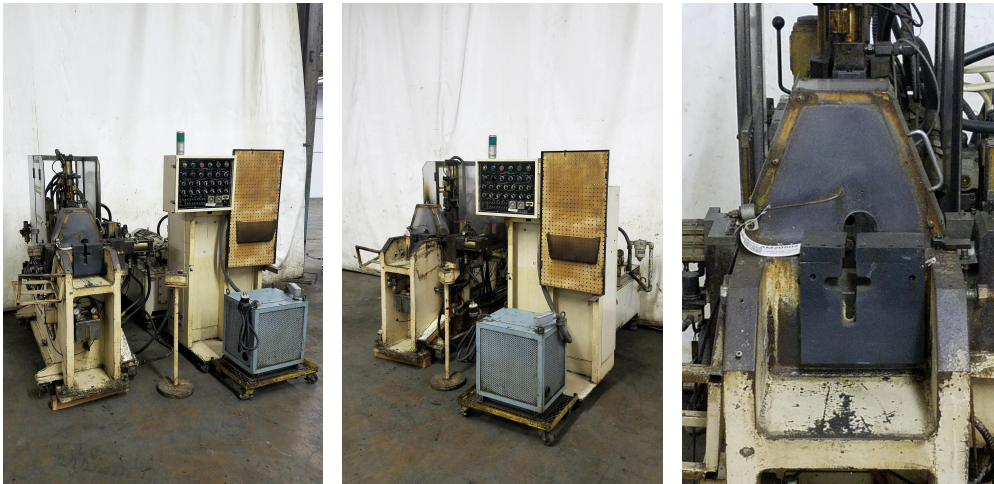
1" (25mm) Taisei #PHD-254DT Tube End Former with Secondary Clamps
